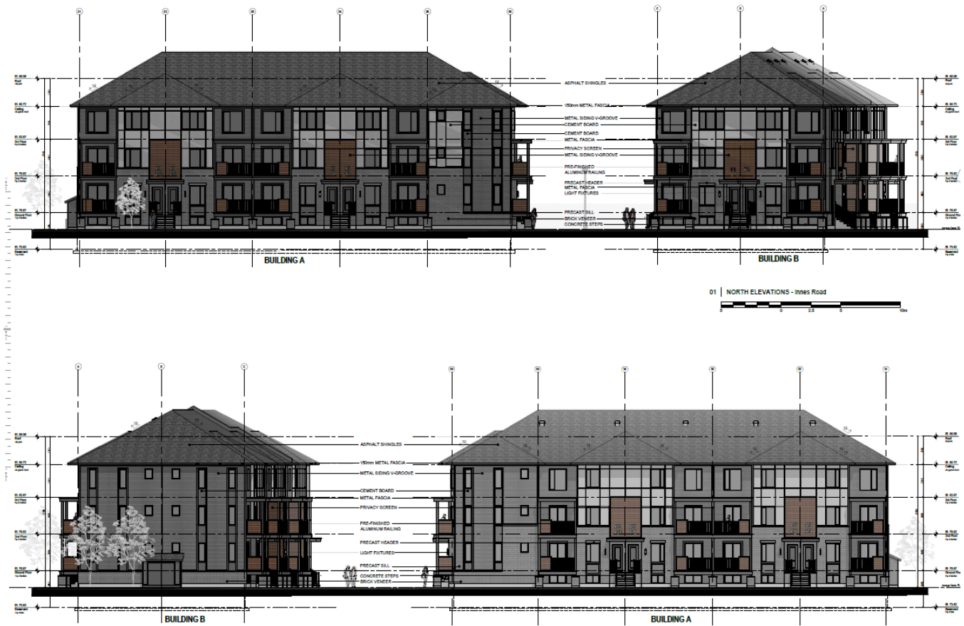
Figure 9: Building elevations facing the front of the buildings (top images) and the rear (bottom images).
