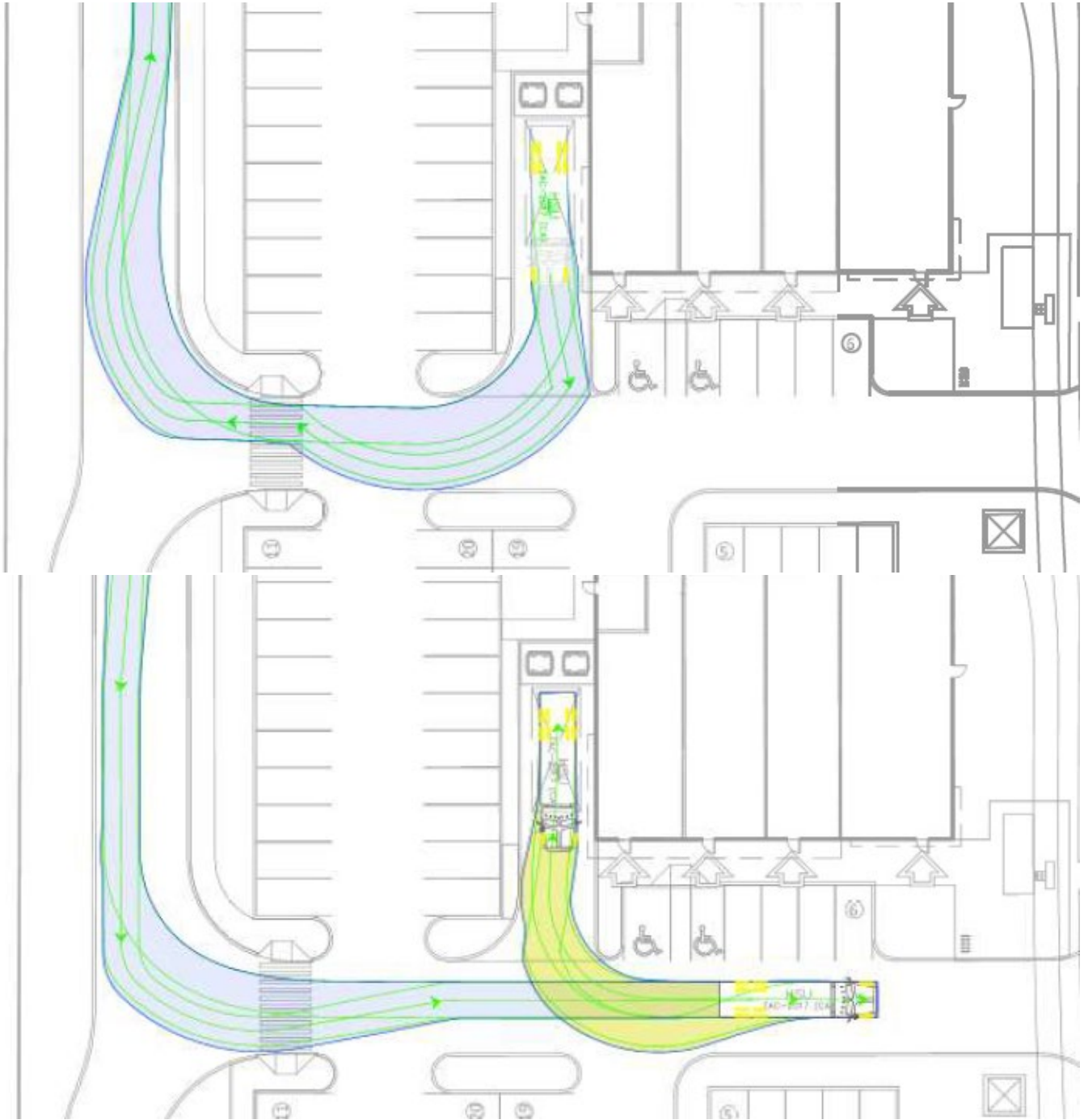
Figure 11: Exit (top) and entry (bottom) turning templates from the proposed CRU loading space on the subject property (Transportation Impact Assessment, prepared by CGH Transportation, dated March 25)
