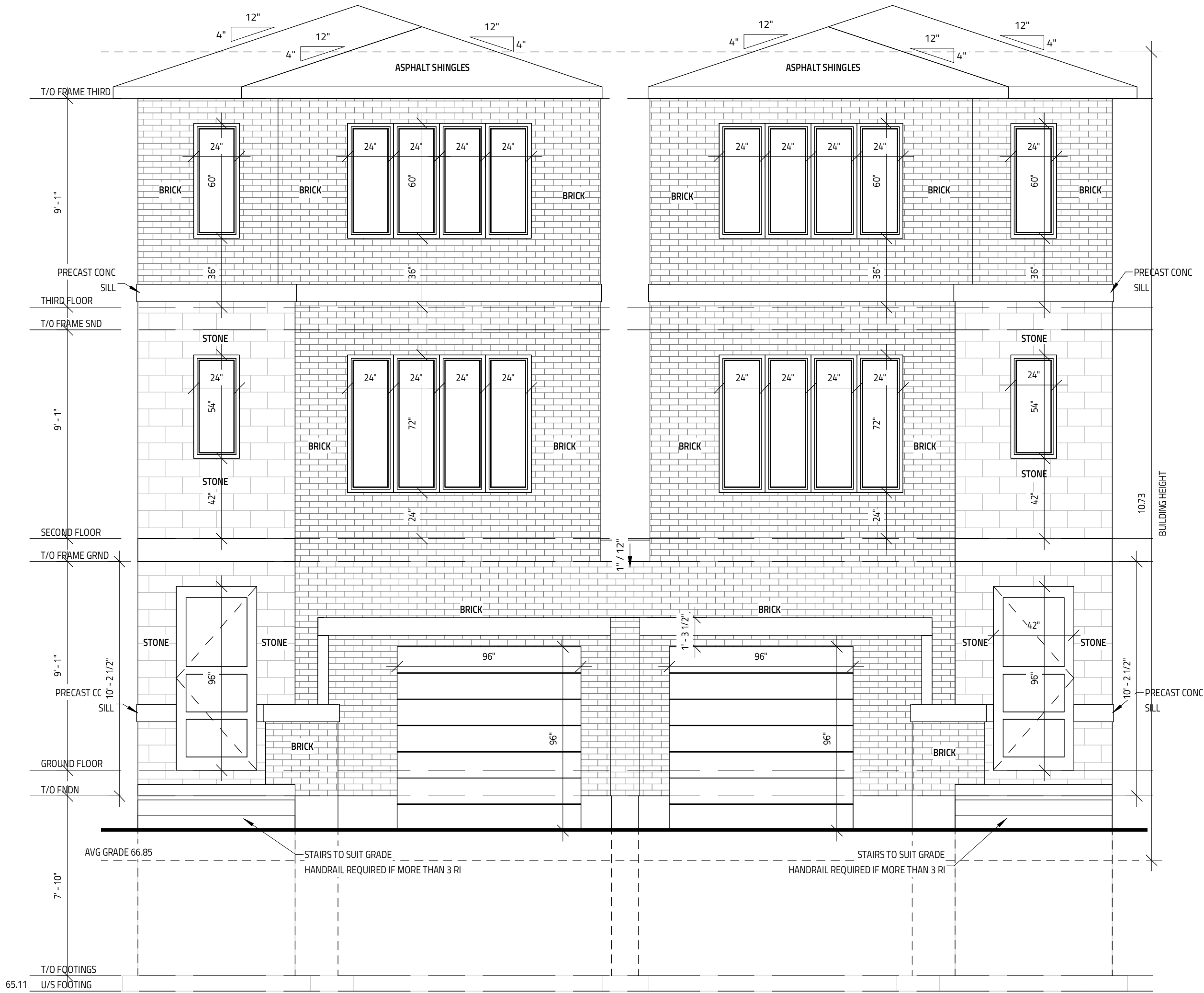
1 FRONT ELEVATION SCALE: 1/4" = 1'-0"
