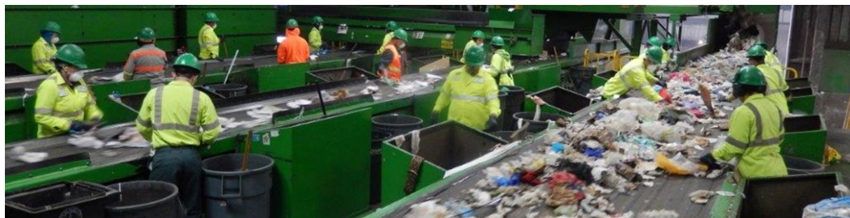
Photo: Manual Sorting Line, Greenwaste Materials Recovery Facility, San Jose, California, USA.
