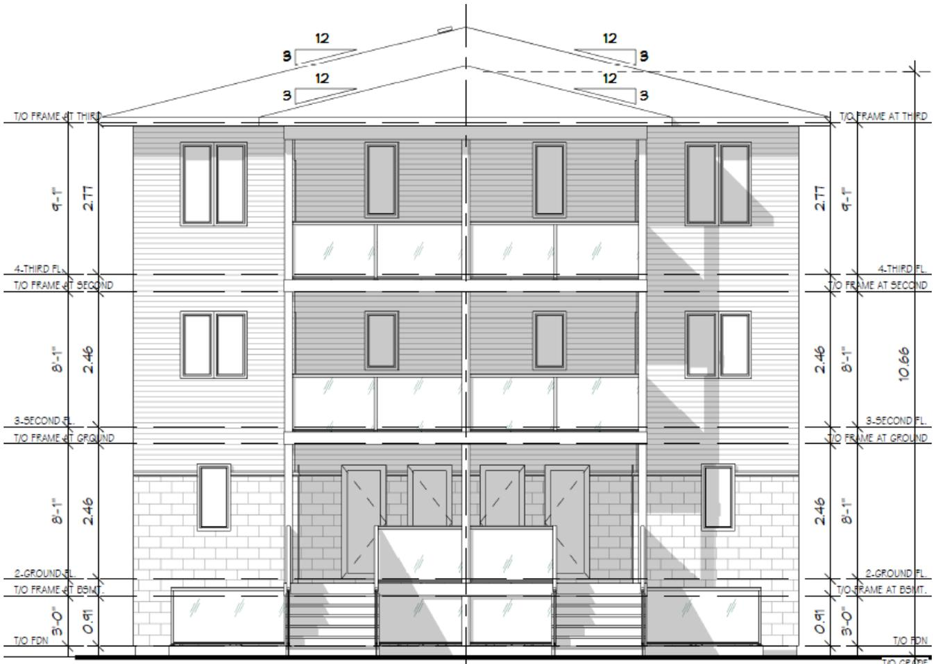
Figure 4: Front elevation of proposed building.
