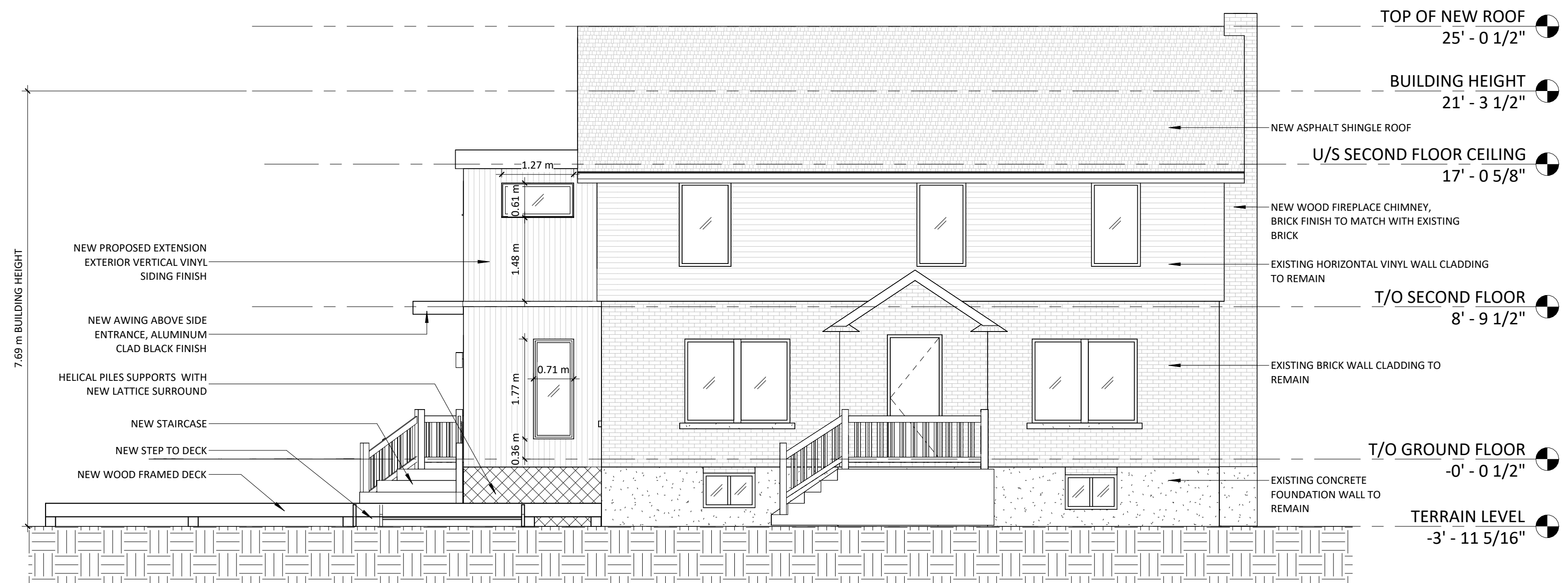
1 ELEVATION AT WEST FACADE A3 3/16" = 1'-0"
