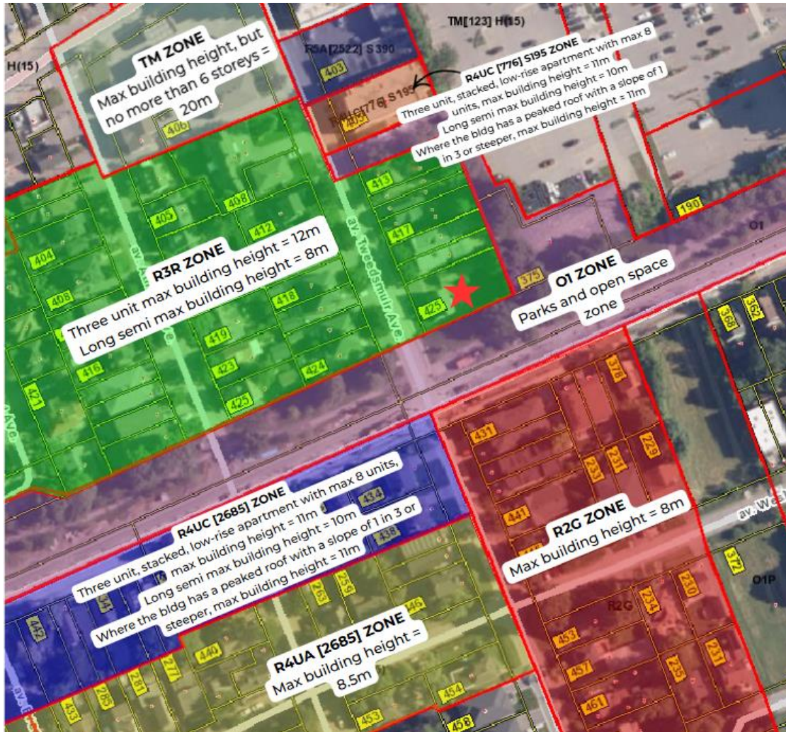
Figure 4. Height Restrictions by Surrounding Zone
