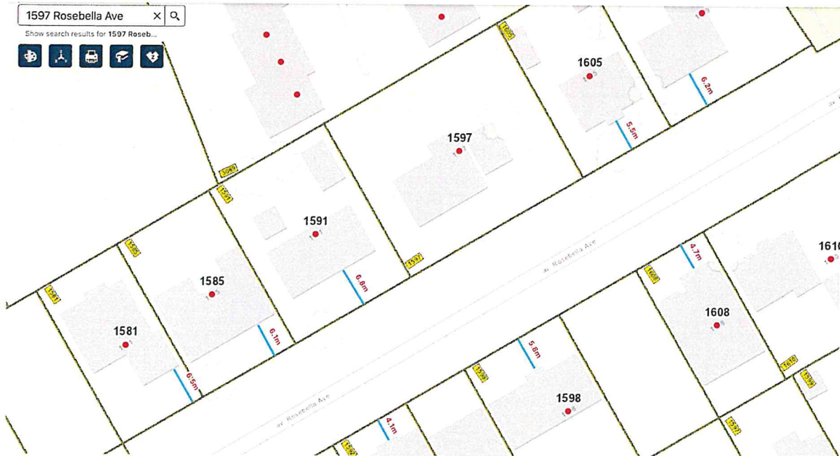
Figure 16: Front yard setback of surrounding property is between 4 - 6 m. The proposed lots have front yard setback of 5 m
