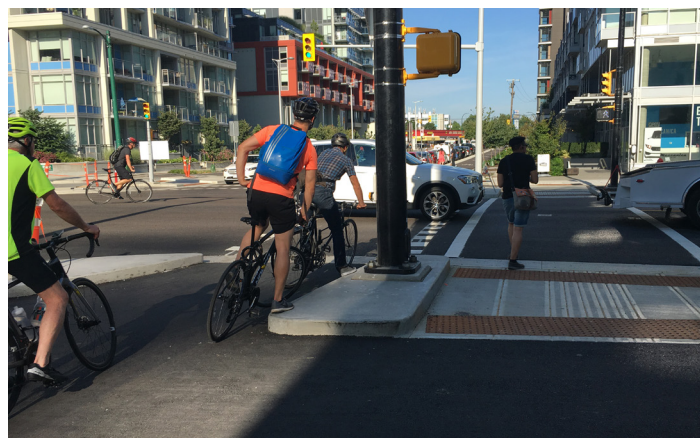
Image 6.8. Vancouver protected intersection with raised island and traffic infrastructure
