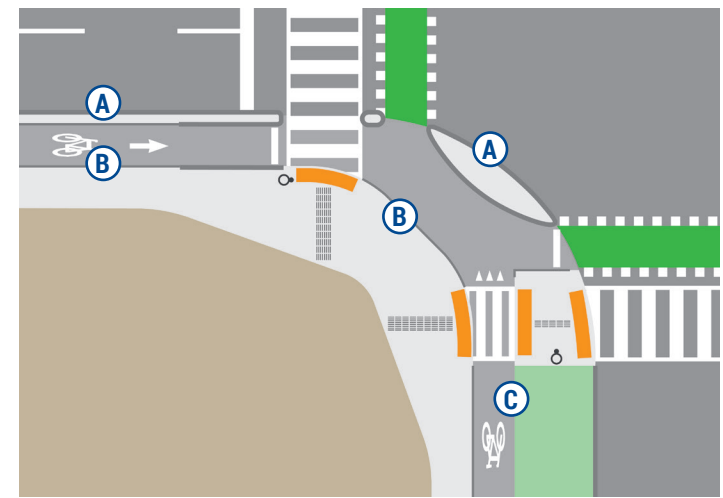
Figure 6.4. Hybrid protected corner showing relative curb heights
