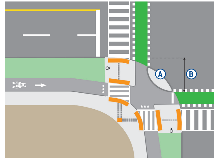
Figure 5.4. Standard protected corner with 10.0 m radius showing 5.0 m crossride setback
