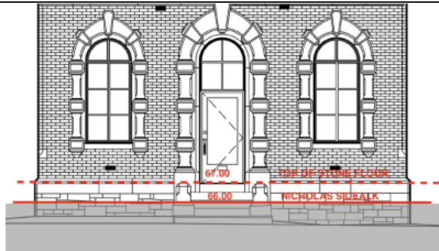
Figure 4: The red markers indicate the relationship of the building to Nicholas Street with a reduced grade difference. The shading at the base of the drawing indicates the new ground level.
