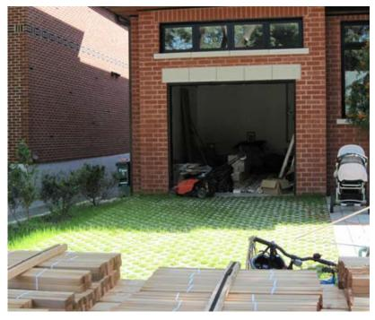
Figure 29: Turf block provides a stable base for parking while increasing on-site infiltration of surfacewater.
