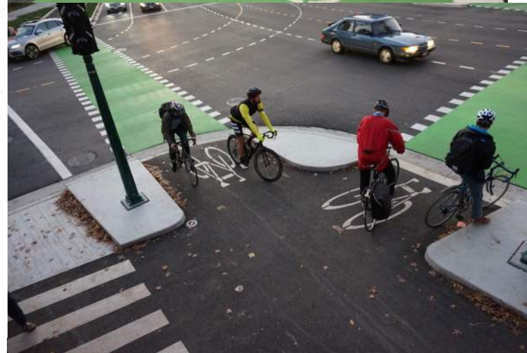
Figure 5.4. Standard protected corner with 10.0 m radius showing 5.0 m crossside setback
