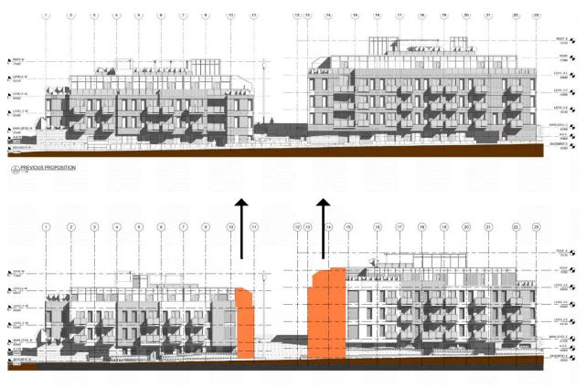
Figure 31: Elevations illustrating the reduction on massing with the revised proposal
