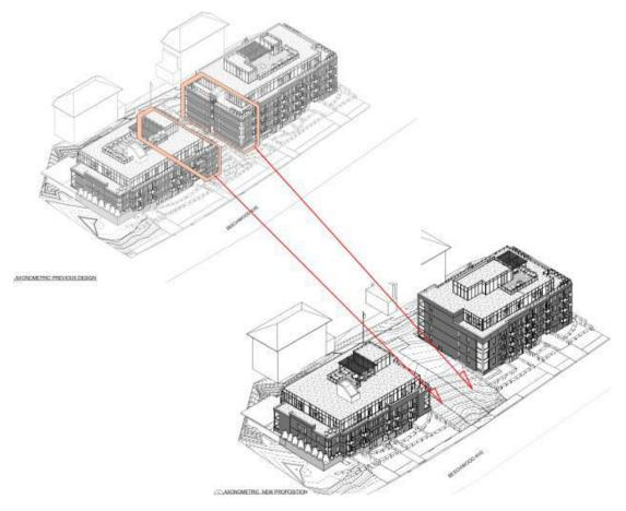
Figure 19: As the illustration shows the revised design significantly reduces the footprint of the previous concept to allow for increased open space adjacent to the proposed buildings. The massing is further reduced by shrinking the floor area of all storeys, accordingly, including the corresponding stepping of upper floors. The visual link between Beechwood and Acacia is an important vista that ismaintained.
