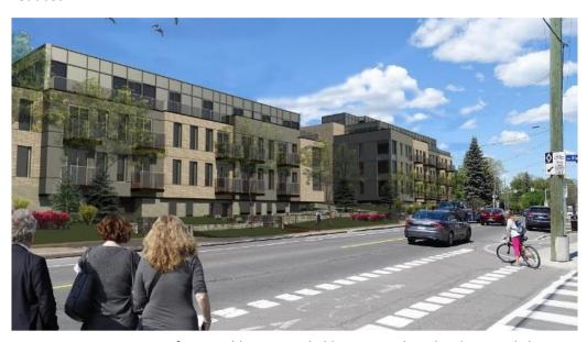
Figure 21: Using a variety of compatible exterior cladding materials and architectural elements arranged to break up the façade into vertical elements along with a streetscape that maintains individual entrances and driveways to evoke the former pattern of development.
