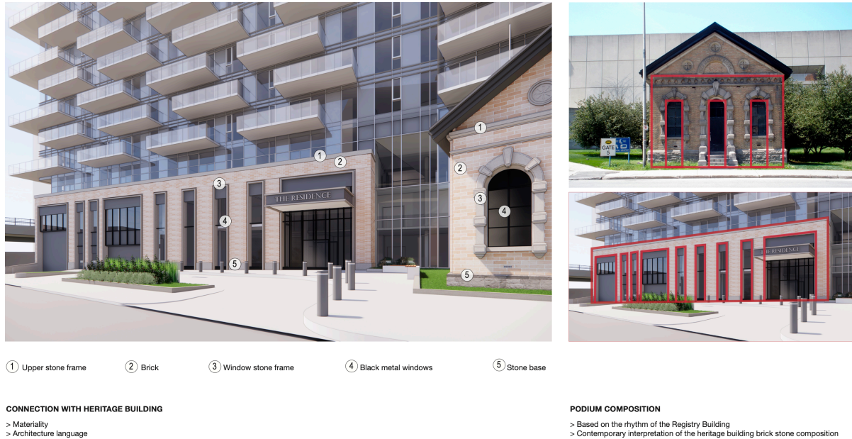
Figure 11: Relationship to Heritage - Given the differences in scale, it is considered key to its visual compatibility that the materiality, and colour of the base of the high-rise act as a backdrop to the CRO without overwhelming it. Introducing the salmon yellow brick with the limestone trim and the black metal into the new development's podium successfully references defining features of the CRO. Source: Zeidler/Neuf 2022.
