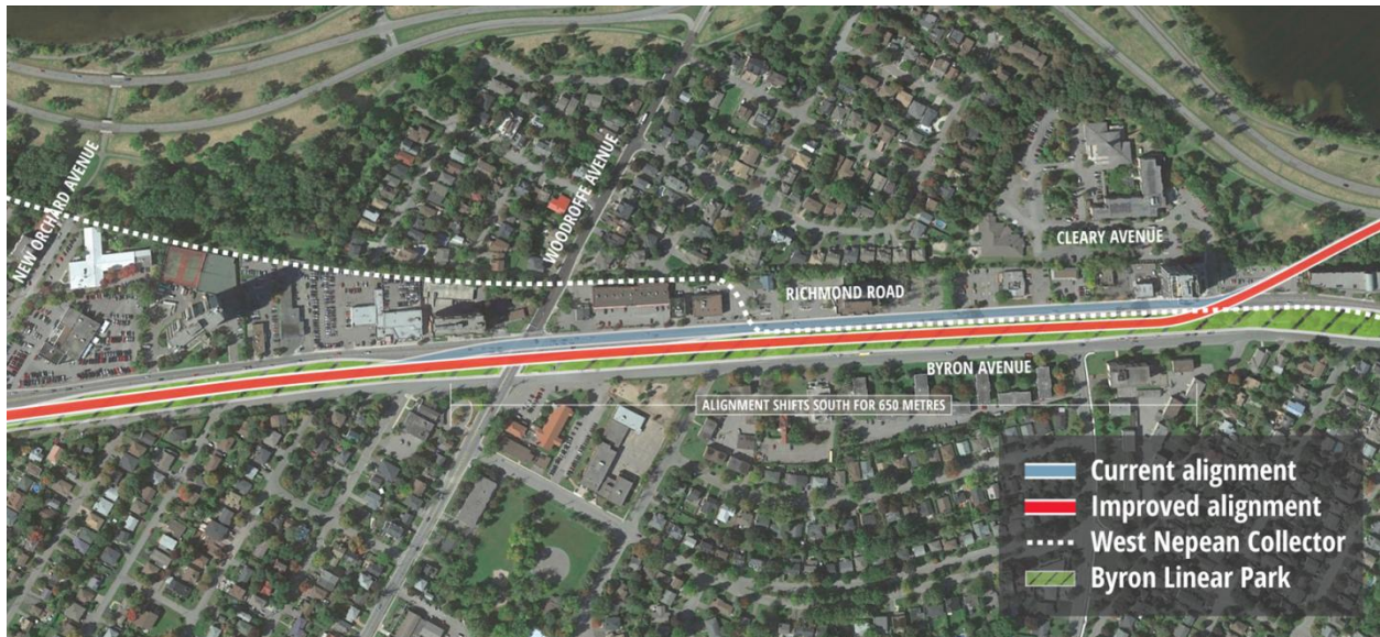
Figure 1: Alignment Improvement at Richmond Road
