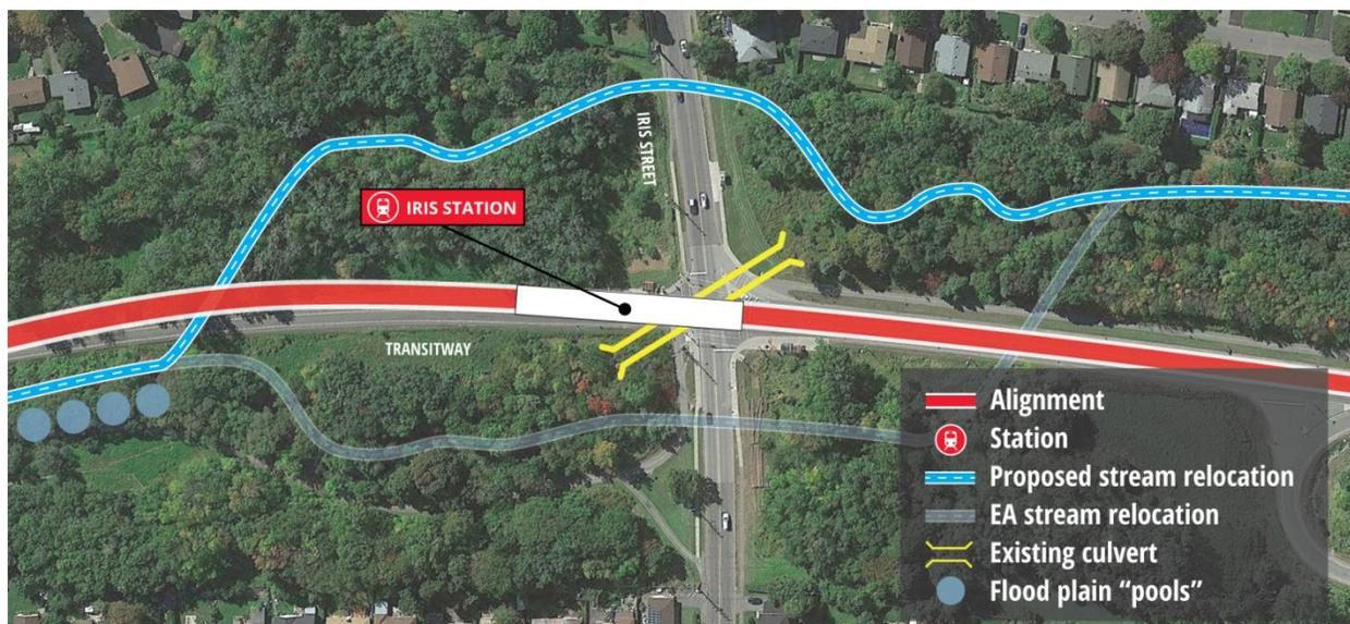
This alternative Pinecrest Creek relocation can be implemented at a comparable capital cost while reducing maintenance costs over the long term. The alignment of the creek will meander by 40 metres over the relocated length of the creek. This will mitigate the impacts of the new creek alignment and improve the health of Pinecrest Creek by minimizing erosion, reducing water velocities, and improving water quality.
