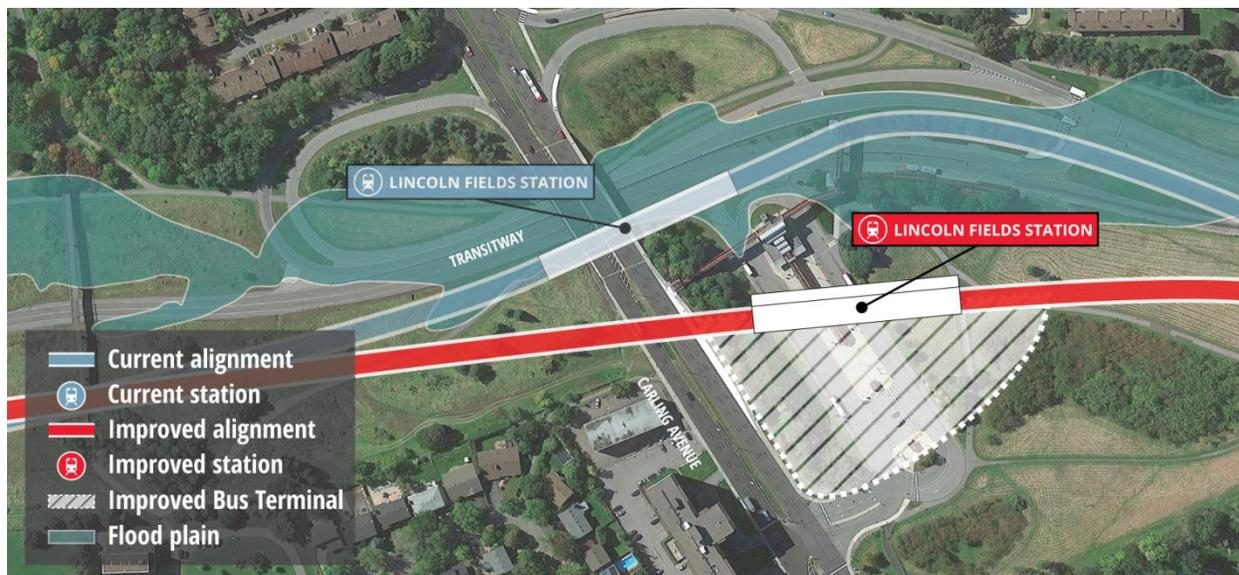
The recommended alignment can be implemented at a comparable cost. In addition, the alignment change would include a new Lincoln Fields Station, a new LRT tunnel under Carling Avenue and a new fare-paid bus terminal, reoriented to provide improved station integration with the transit network. Staff undertook a noise and vibration analysis which indicated that with a standard noise wall on the east side of the new bus
