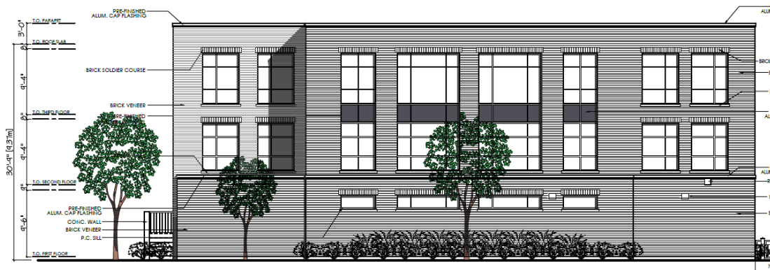
BUILDING 1 - REAR (WEST) ELEVATION SCALE: 1:150
