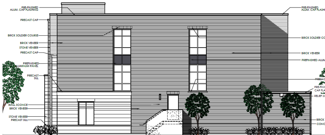
BUILDING 1 - NORTH ELEVATION SCALE: 1:150
