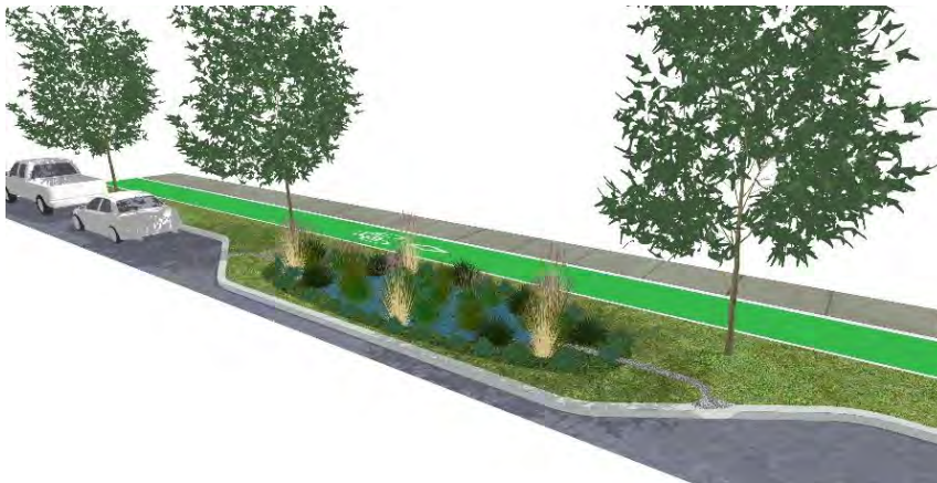
Figure 22 Bulb-outs can provide added space for bio-swales
