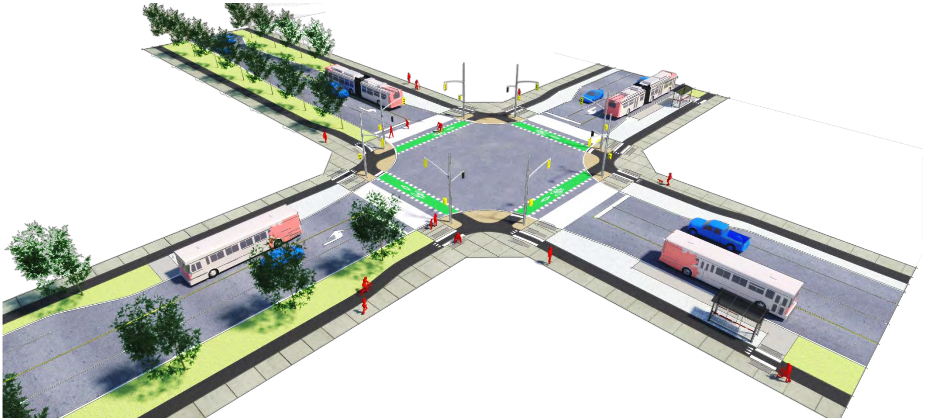
Figure 24 A protected intersection provides separation and clarity of space for all users
