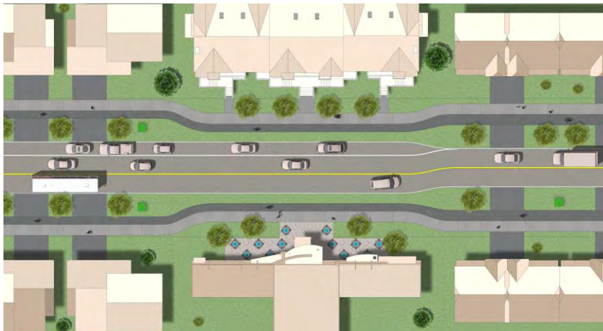
Figure 14 Various cross-section designs can be used along a corridor to respond to the land use context and the transportation functions (not to scale)
