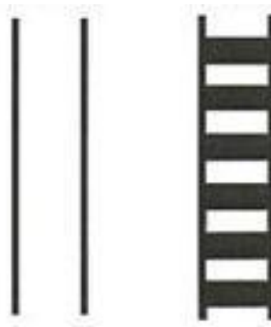
Figure 6 - Crosswalk pavement markings
