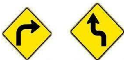
Figure 11 - Curve warning signs
