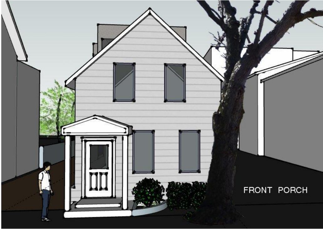
Front elevation showing a proposed porch addition
