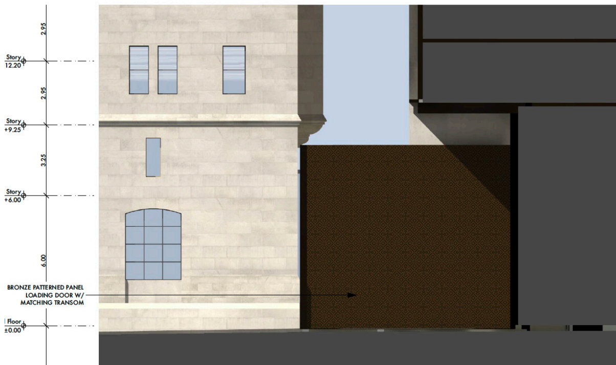
12. Detail of the loading area at the east elevation of the east pavilion (Source: architectsAlliance).
