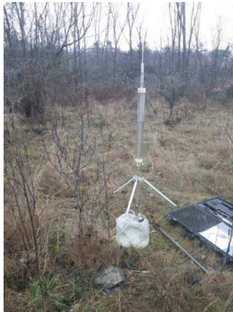
Figure 5: Guelph Permeameter setup in the field. Flexible water reservoir and hand auger in the foreground.
