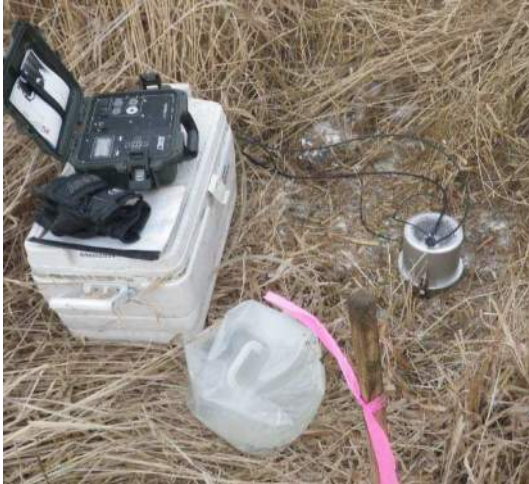
Figure 2: Dual-Head Infiltrometer Setup, control unit shown on the left, flexible water reservoir near the bottom and DHI unit setup on the right side of the image.
