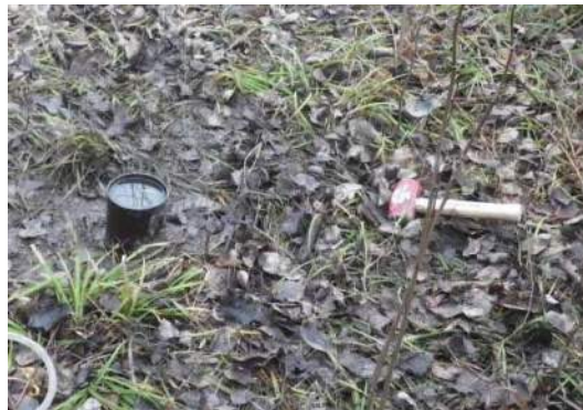
Figure 4: Single Ring Infiltrometer Setup, 11 cm diameter steel ring shown on the left of the image, failing head test in progress with water near the ring top.
