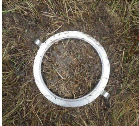
Figure 3: DHI cylinder installed at the ground surface (cylinder penetrates to 5 cm deep), prior to attaching the top of the unit and starting a test.
