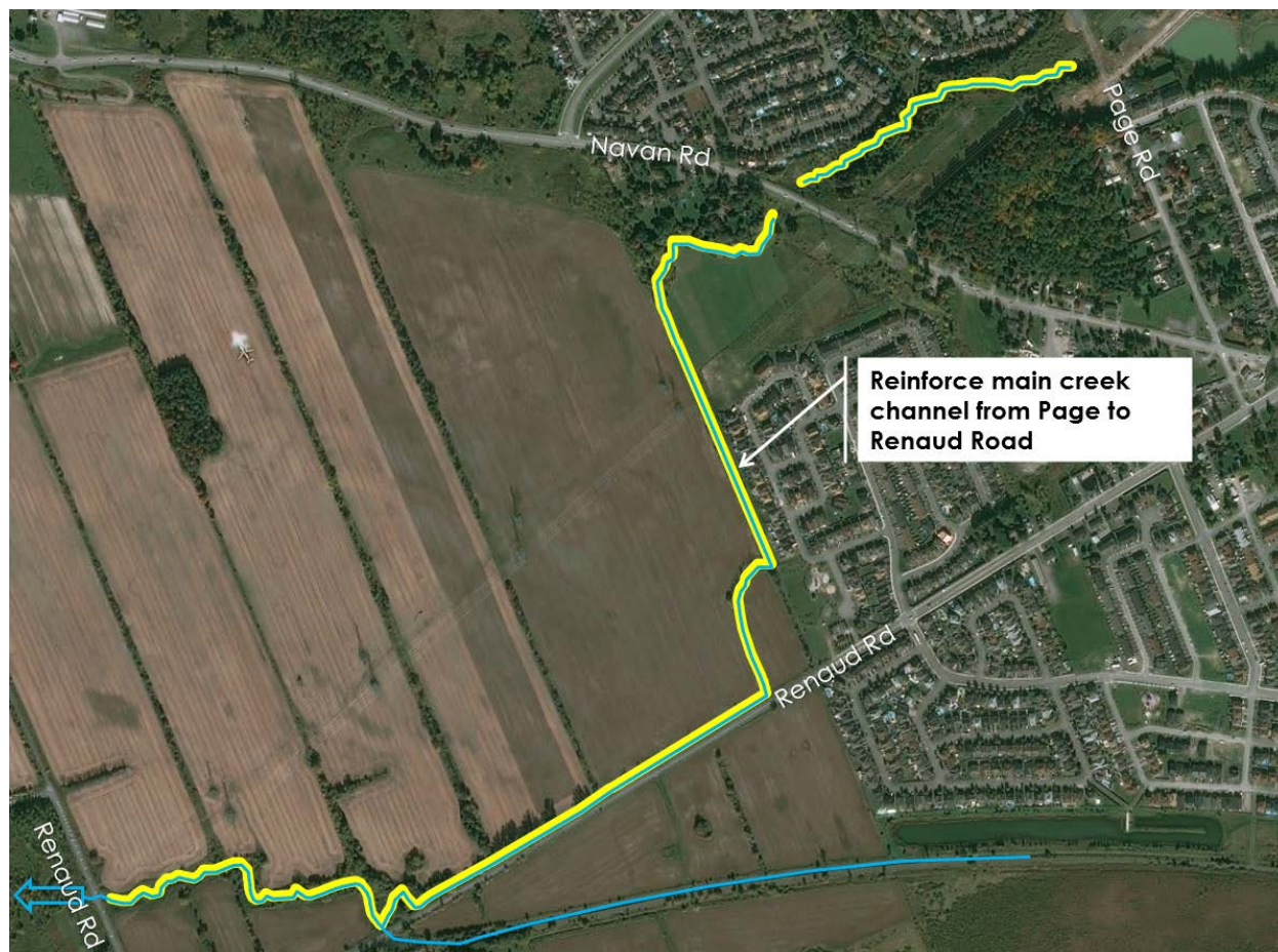
Figure 6-13: Reinforce Existing Channel Approach
