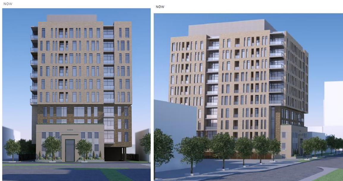
Figure 4. An elevation and a view looking west illustrate the new midrise apartment with the front portion of the original building serving as the main entry and building foyer. Source R Lahey Architect 2020.
