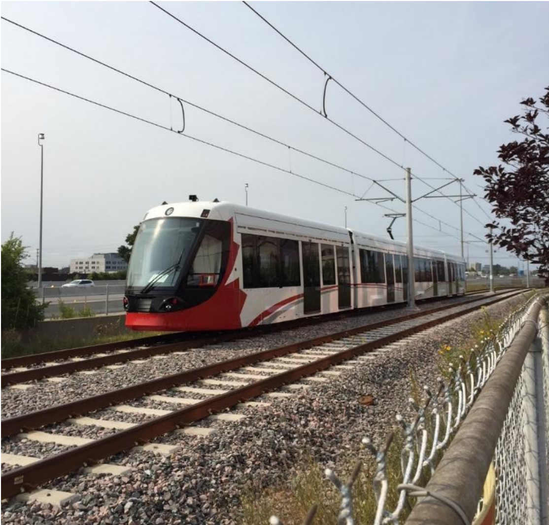
Figure15: Fully Segregated Rail (Ottawa's LRT)
