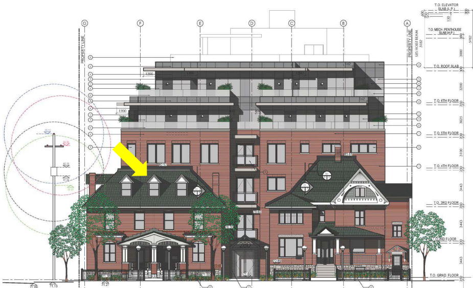
Figure 11: East elevation (O'Connor Street elevation) of the proposed development, illustrating the addition of a new dormer at 280 O'Connor (David Blakely Architect Inc.)
