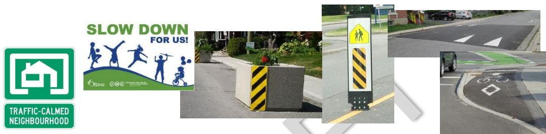
Figure 1 - Traffic Calming Measure Examples
