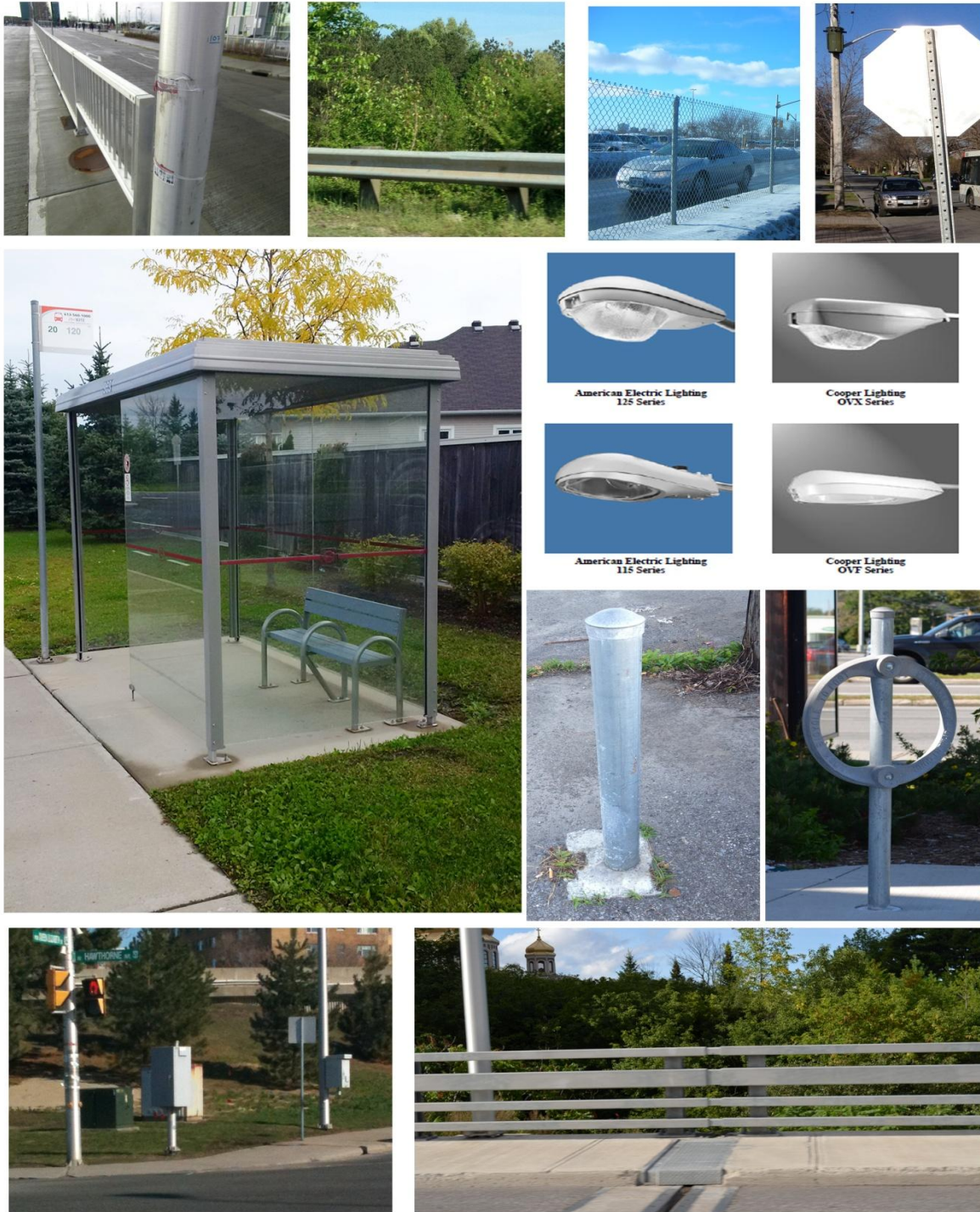
Figure 1 - Typical (standard) right-of-way assets
