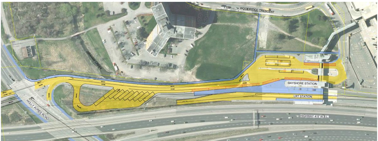
Figure 35: Diagrammatic plan view of Bayshore Station showing LRT platforms, bus platforms, bus staging area and Holly Acres Road intersection to West Transitway Extension
