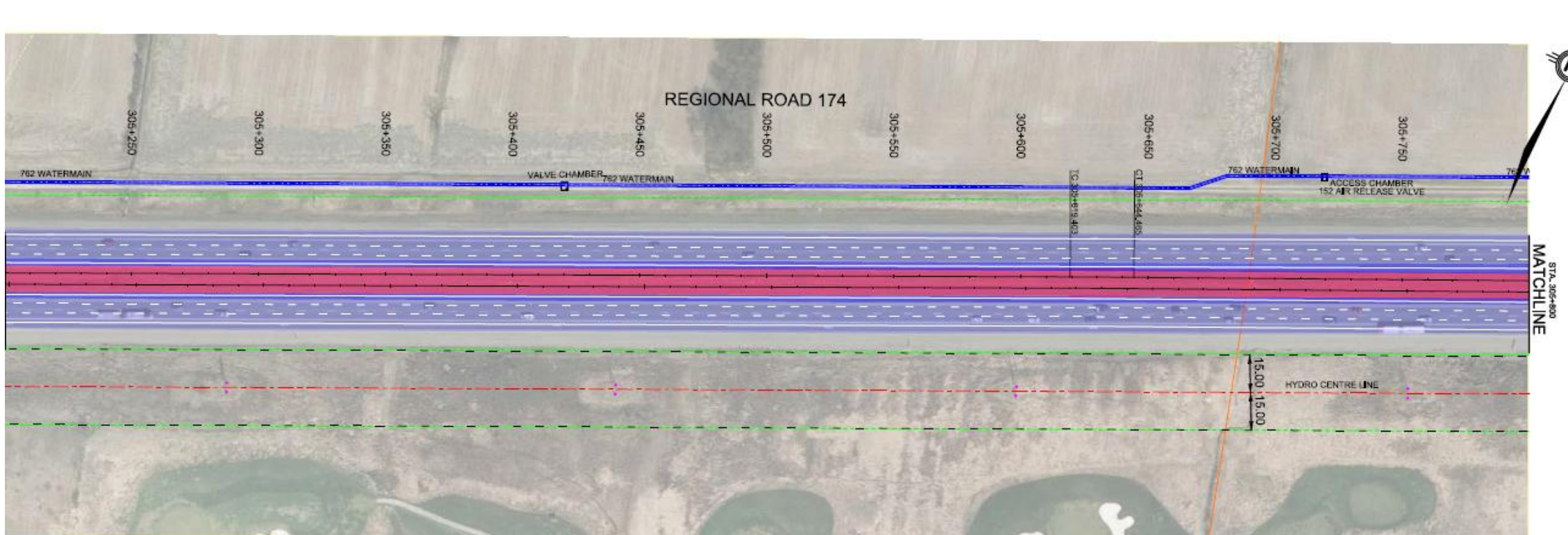
Figure 26: LRT track and highway widening through greenbelt
