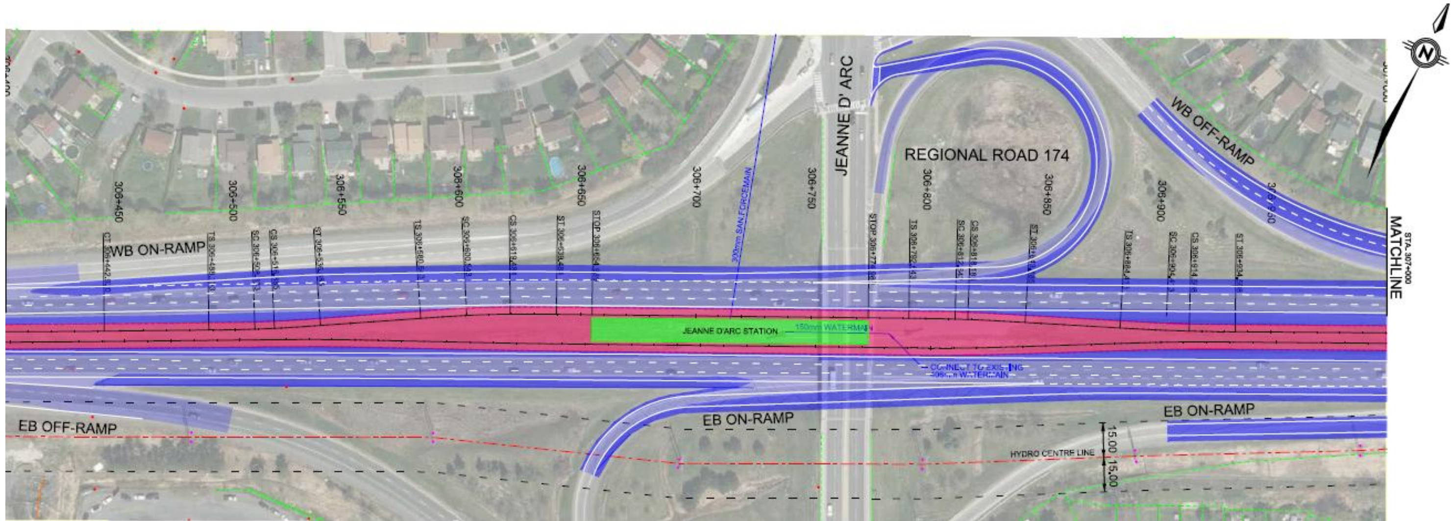
Figure 28: Jeanne D'Arc Station, highway widening and ramp modifications
