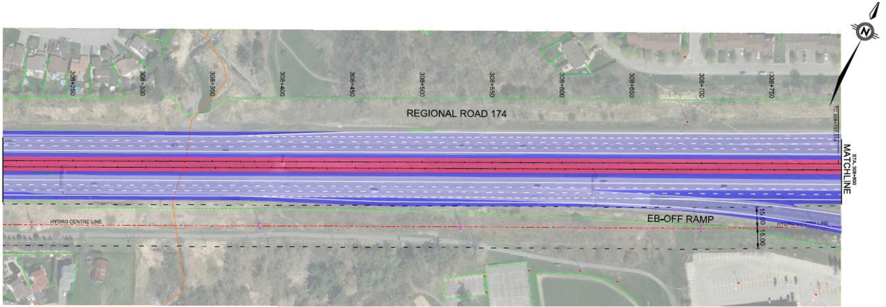
Figure 31: LRT track and highway widening near Taffy Lane
