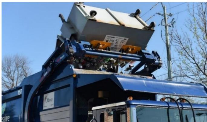
Both the containers and carts are collected using a front-end loading truck.
