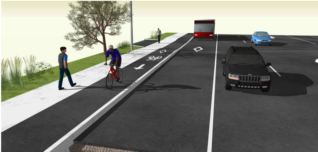
Figure 2- Transit Lanes with raised Cycling Track.
