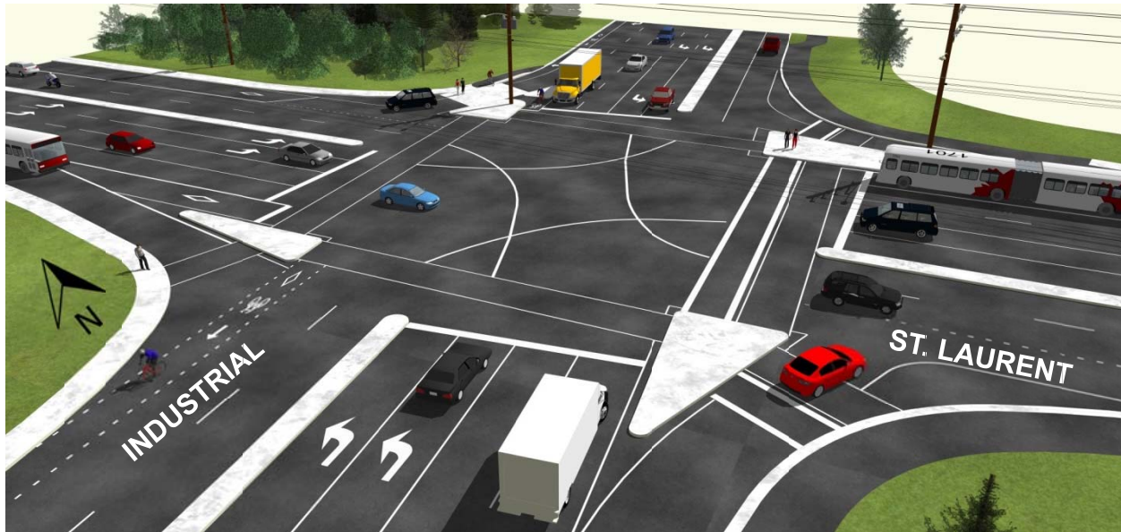
Figure 6-3: Proposed configuration at Innes Road / Industrial Avenue / St. Laurent Boulevard intersection (traffic signals and lighting not shown for clarity)
