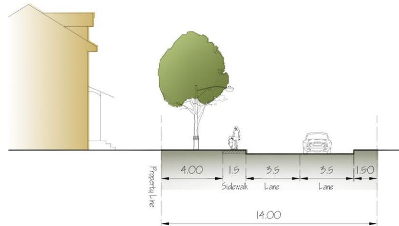
FIGURE 12: Single Loaded Road Cross Section (14.0m)
